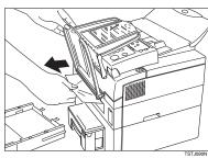
**2** Push down the paper so that the base plate locks into place.
